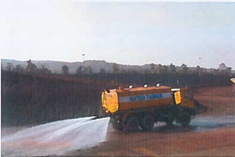
SPRINKLING THROUGH WATER TANKER
